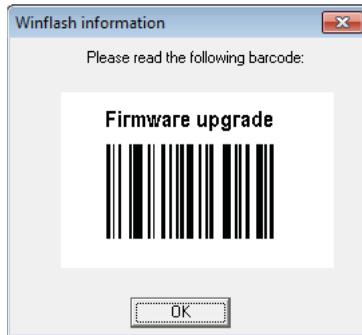
The scanner emits two beeps and two green flashes to indicate a good configuration bar code read and then blinks with a regular red blink.
