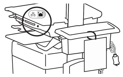
**Ethernet:** This cable runs from the side of the enclosure to your computer to allow network connection from the ethernet port on the outside of the enclosure.
