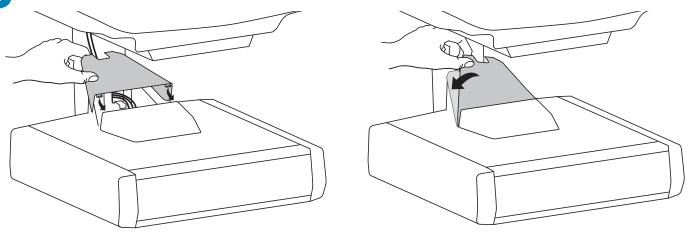
To unlock the storage drawer, turn key counter clockwise 1/4 turn.
