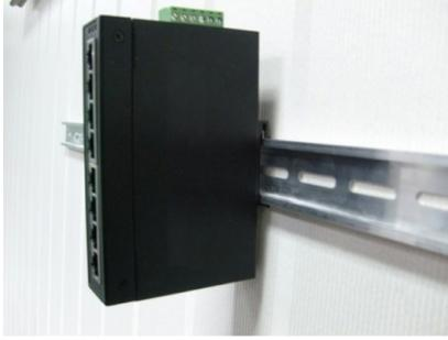
**Figure 6:** Industrial Equipment installed in DIN-Rail mount.
