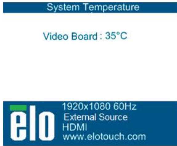
Example of OSD showing the Video Board Temperature
