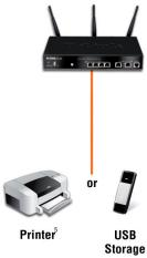
Supports one (DSR-250N/500/500N) or two (DSR-1000/1000N) USB 2.0 devices to extend functionality via D-Link's SharePort feature.
