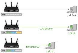
D-Link Green Ethernet detects link status and cable length and adjusts power usage accordingly.
