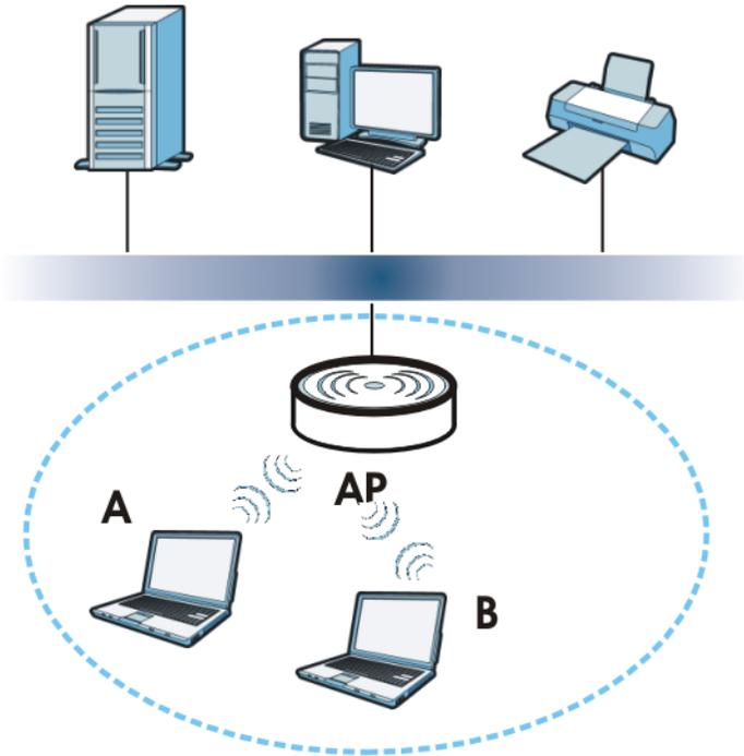
The wireless network is the part in the blue circle. In this wireless network, devices **A** and **B** are called wireless clients. The wireless clients use the access point (**AP**) to interact with other devices (such as the printer) or with the Internet. Your NBG-418N v2 is the AP in the above example.
