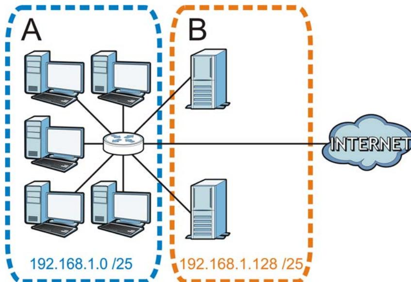
In a 25-bit subnet the host ID has 7 bits, so each sub-network has a maximum of  $2^7 - 2$  or 126 possible hosts (a host ID of all zeroes is the subnet's address itself, all ones is the subnet's broadcast address).
