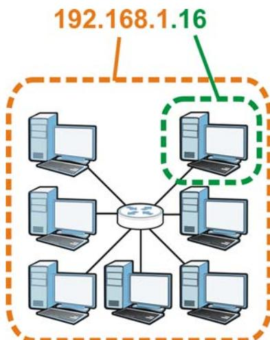
How much of the IP address is the network number and how much is the host ID varies according to the subnet mask.
