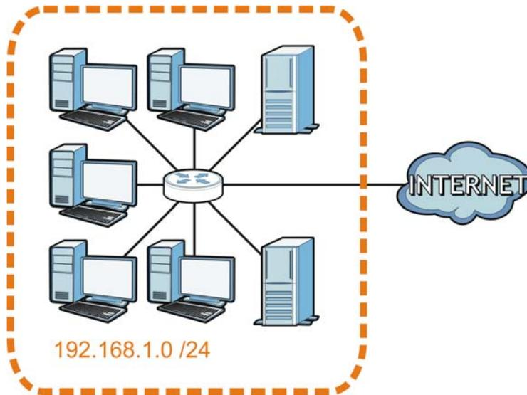
You can “borrow” one of the host ID bits to divide the network `192.168.1.0` into two separate sub-networks. The subnet mask is now 25 bits (`255.255.255.128` or `/25`).
