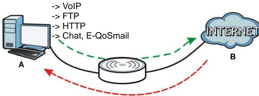
You can allocate specific amounts of bandwidth capacity (bandwidth budgets) to individual applications (like VoIP, Web, FTP, and E-mail for example).
