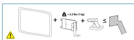
CAUITON: Make sure you know the max. weight capacity of your mounting solution before attaching the scanner shelf. Include the weight of your monitor, scanner shelf, scanner base and scanner: when figuring mounted weight on your mounting solution. Failure to follow this Caution may lead to equipment damage and/or personal injury.
