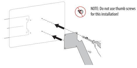
Attach part "1A" to VESA plate at the back of your display. Insert two of the provided M4x14mm phillips screws through the bracket, the VESA plate and display.
