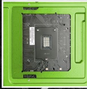
Installation Opening for CPU Coolers
