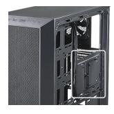
SSD can also be installed behind the motherboard tray
