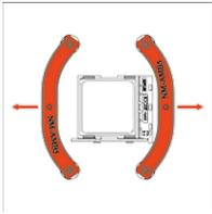
**Caution:** Gently tighten the screws until they stop, but don't use excessive force (max. torque 0.6 Nm).
