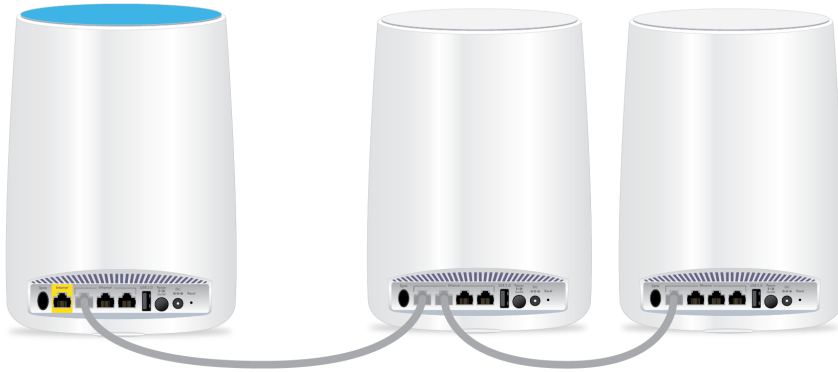
Figure 14. Satellite 1 connected to router and satellite 2 connected to satellite 1
