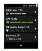
The connections screen appears. A flashing icon means the device is searching.
