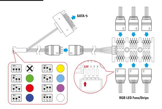
To illuminate RGB LED fans and strips on motherboards without a 12V-G-R-B connector, connect the manual color control as shown. The color of the RGB channels can then be selected via the DIP switches.
