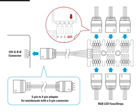
The 6-port RGB hub is self-adhesively attached to the case interior and then connected to the mainboard's 12V-G-R-B connector. When connecting any elements, make sure that the 12V contact and the arrow on the corresponding connector are facing each other as shown.
