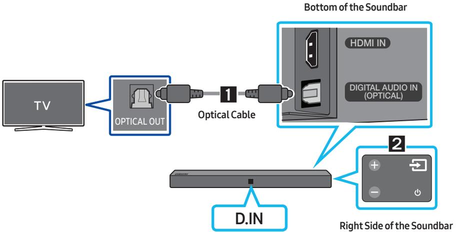
1. Connect the **DIGITAL AUDIO IN (OPTICAL)** jack on the Soundbar to the **OPTICAL OUT** jack of the TV with a digital optical cable.
