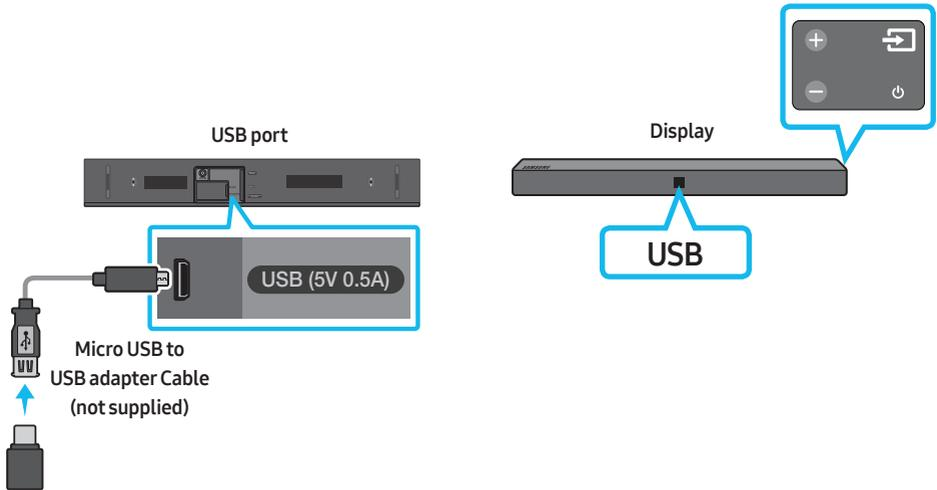
1. Connect a Micro USB to USB adapter cable with a male USB 2.0 Micro USB plug (Type B) on one end and a standard female 2.0 USB jack (Type A) on the other end to the micro USB jack on your Soundbar.
