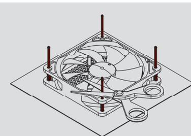
If the long ends of the mounts are in the way, you can use scissors to cut them after installation. Note that this will then make them difficult to reinstall in the future.
