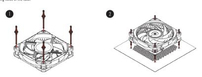
If the long ends of the mounts are in the way, you can use scissors to cut them after installation.
