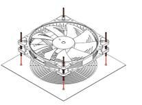
If the long ends of the mounts are in the way, you can use scissors to cut them after installation.
