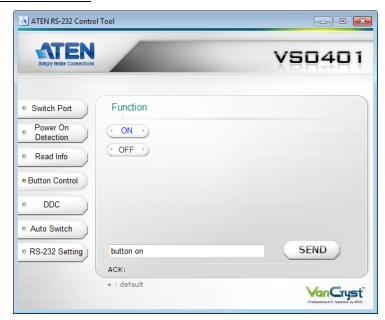
The Button Control page allows you to secure your device by locking use of the front panel pushbuttons.
