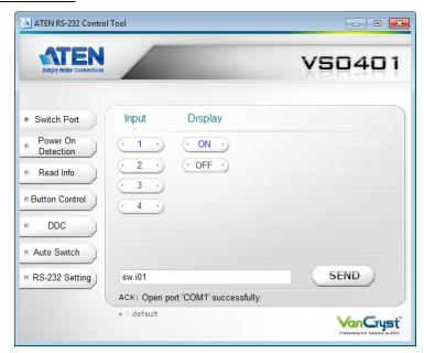
The Switch Port page is used to connect the Video/Audio sources to the display port, and to power on/off the display.
