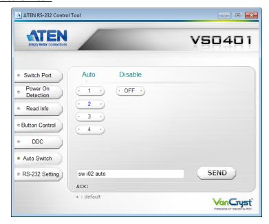
The Auto Switch page is used to enable Auto Switching for a port, or to disable Auto Switching. Auto Switching places priority on a port so that when a source is connected to that port the VS0201 / VS0401 automatically switches to it, and the port can not be changed until the source is unplugged or auto switching is disabled.
