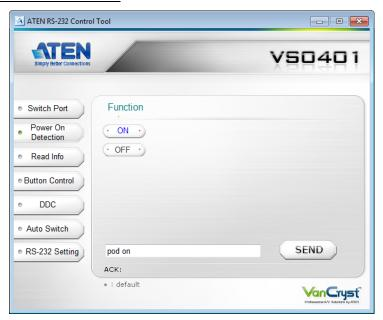
The Power on Detection page is used to enable or disable the Power on Detection feature. Power on Detection is used to automatically switch to the next port with a powered on device, when the current port device is powered off.
