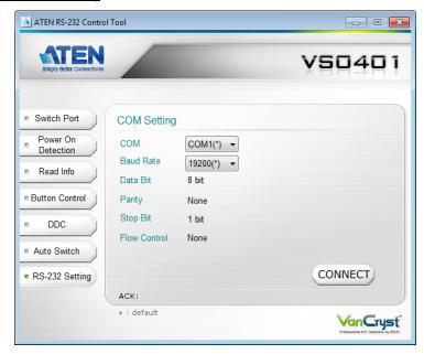
On the RS-232 Settings page, the serial port should be configured as follows:
