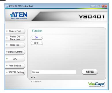
The DDC page is used to enabled and disable Dynamic DDC. Dynamic DDC is used to monitor the connected display and provide the correct updated EDID information to the source device so that the display is optimized. With Dynamic DDC off, source devices do not receive updated EDID data which can cause display issues. If there is a problem with your display quality, it is recommended that Dynamic DDC be turned off.
