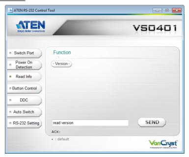
The Read Info page is used to get the VS0201 / VS0401's firmware version. From the Read Info page, the following Functions are possible:
