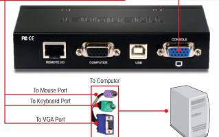
Connect a Cat.5/5e/6 Ethernet cable from the Ethernet port on the Transmitter (local device) to the Ethernet port on the Receiver (remote device).
