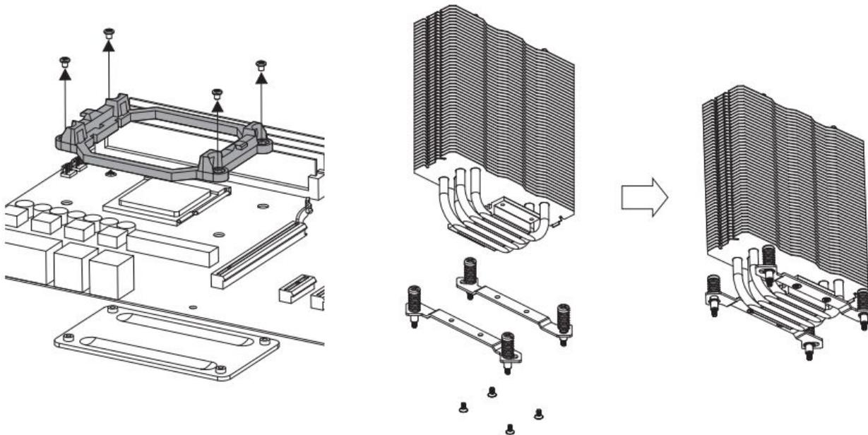
1. Unscrew and remove the standard AMD™ socket bracket (keep the motherboard backplate).
