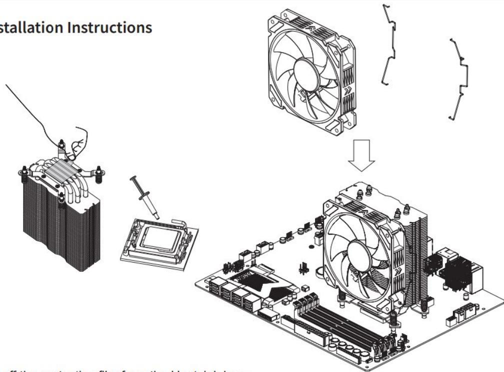
3. Peel off the protective film from the Heatsink base.
