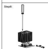
Step 6: Place the heatsink on top of the cpu, and then tighten the hexagonal screws on both ends of the mouting plate.
