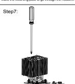
Step 7: Place the heatsink on top of the cpu, and then tighten the hexagonal screws on both ends of the mouting plate. Use the included screw driver to fix the hexagonal screw underneath the heatsink.
