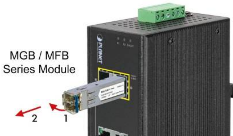
Figure 2-6: Pull Out the SFP Transceiver Module
