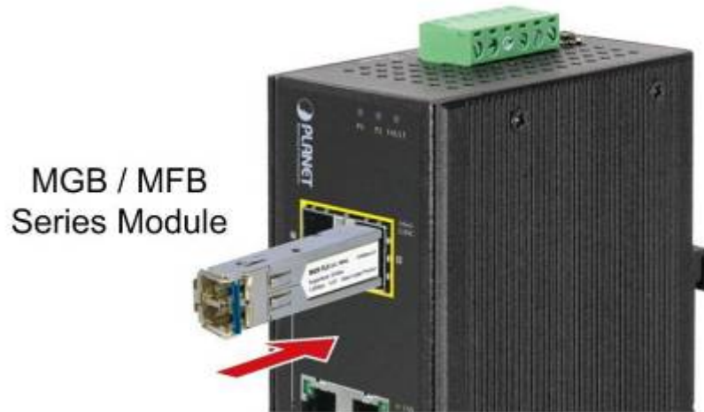
Figure 2-5: Plug-in the SFP Transceiver
