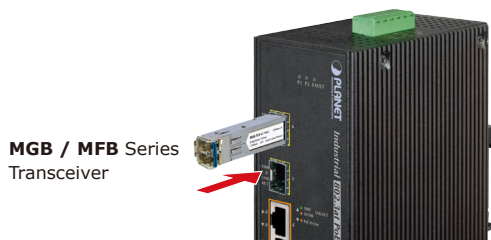
Figure 2-3: Plug-in the SFP transceiver
