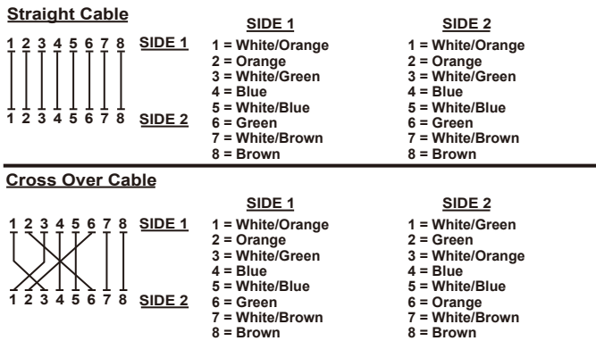
Figure A-1: Straight-through and Crossover Cable
