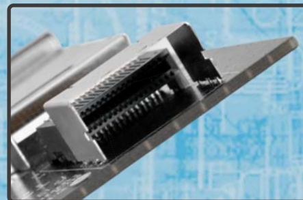
Internal : Mini-SAS SFF-8087 x 1 (to host terminal, e.g. motherboard or Mini-SAS expansion card)
