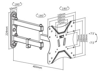
Install the wall plate to the wall
