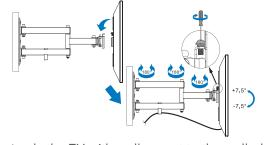
Apply the TV with wall mount to the wall plate
