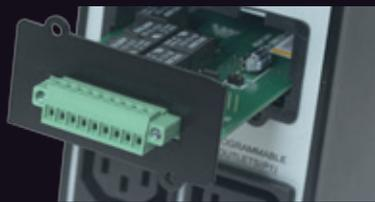
An optional AS400/relay card can be added to the ZINTO for communication with IBM AS400 servers or for integration in industrial switchgear. Dry-contacts (via relay) with the following functions are available on its terminal strip: Normal operation, battery operation, battery voltage low, bypass mode, standby mode, group fault. The UPS can be shut down remotely via an additional input contact.
