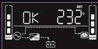
ZINTO's liquid crystal display shows basic information about input and output voltage, frequency, autonomy time and load. The display can be rotated without tools and the installation type of the UPS system can be modified as tower or in rack to make sure it can be ergonomically read.
