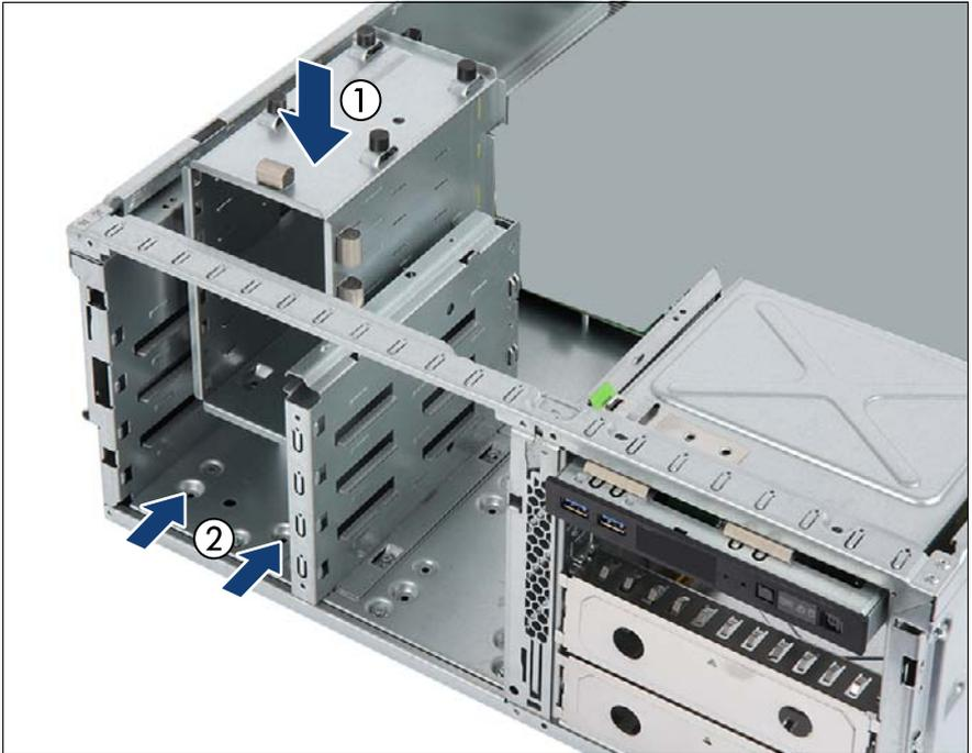
Figure 134: Installing the 2.5-inch HDD/SSD cage
