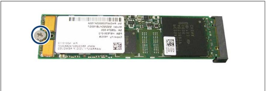
Figure 288: Removing the M.2 SSD (A)
