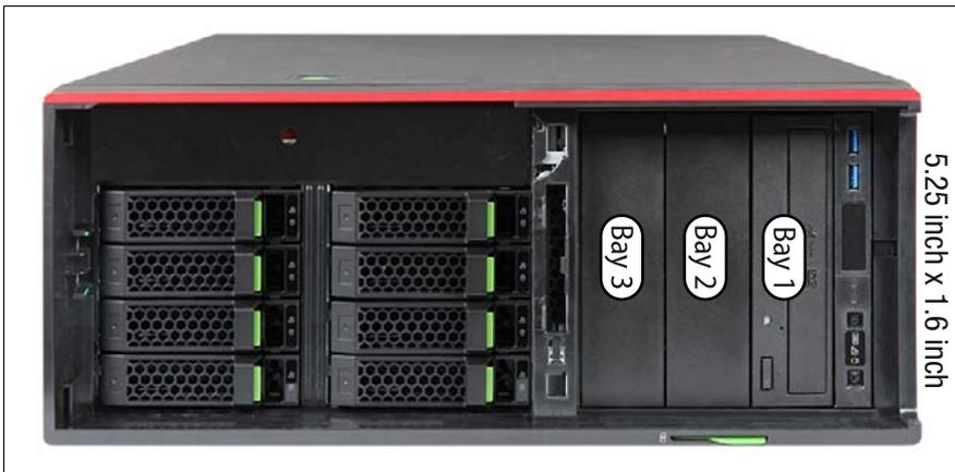
Figure 236: Accessible drives mounting order (floorstand model)
