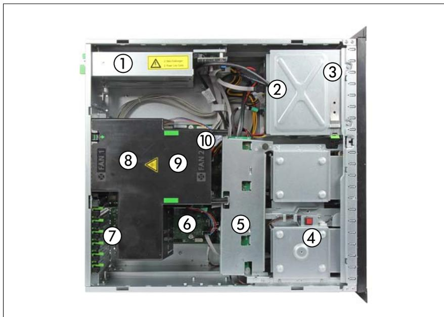
Figure 329: Interior (example: 2.5-inch HDD model, redundant power supply)
