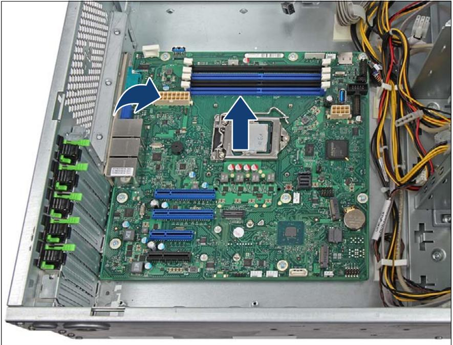
Figure 297: Removing the system board
