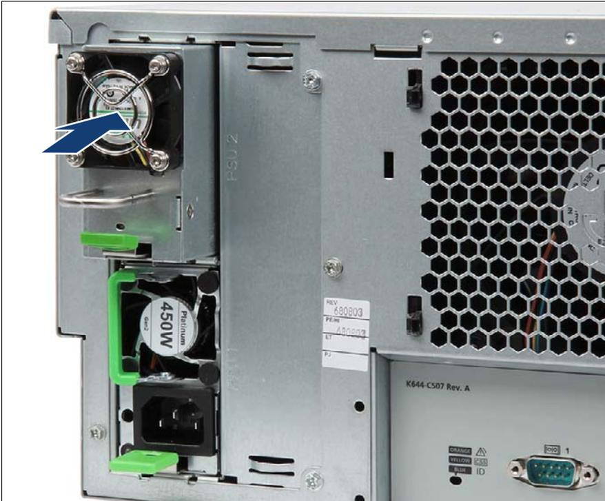
Figure 79: Installing a FJBU
