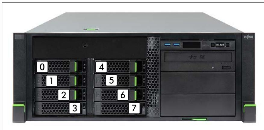
Figure 95: Configuration with up to eight 3.5-inch HDDs
