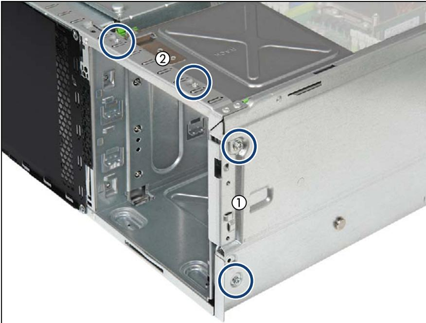
Figure 308: Securing the accessible drive cage (A)
