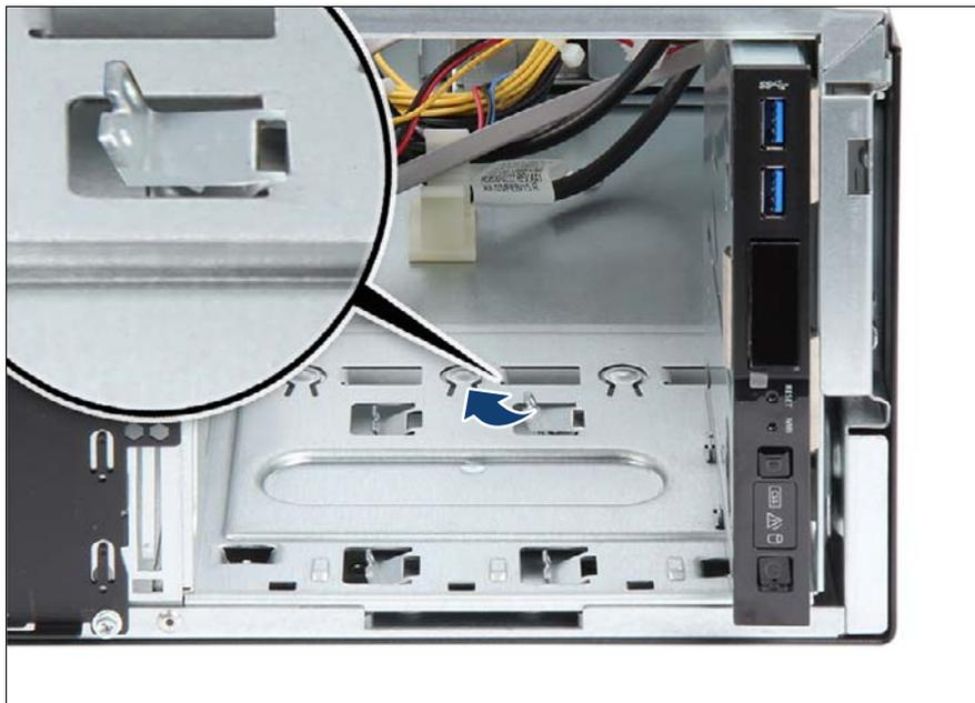
Figure 241: Mounting brackets in right position
