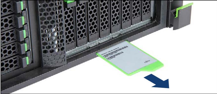
Figure 8: Removing the ID card (rack model)
