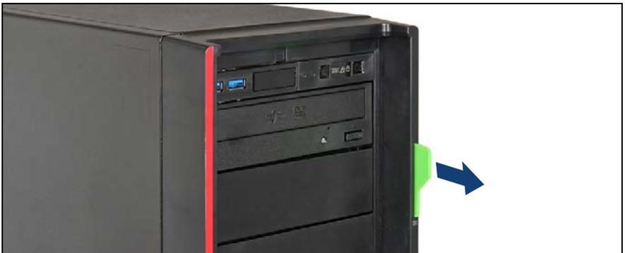
Figure 18: Removing the ID card (floorstand model)
