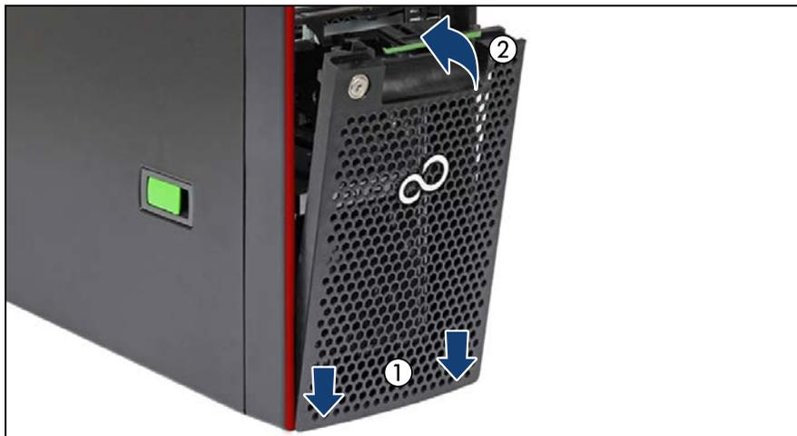
Figure 30: Installing the HDD bay cover
