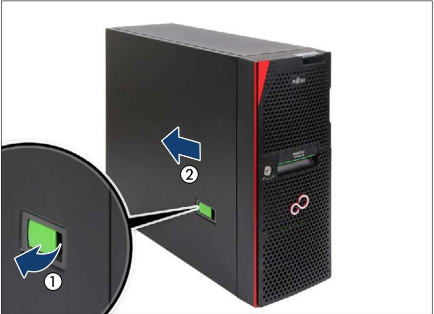
Figure 14: Removing the side cover (floorstand model)
