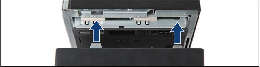
Figure 27: Installing the front cover (A)
