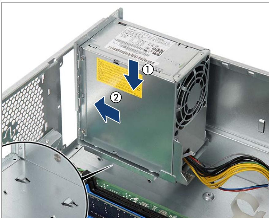
Figure 63: Installing the standard PSU
