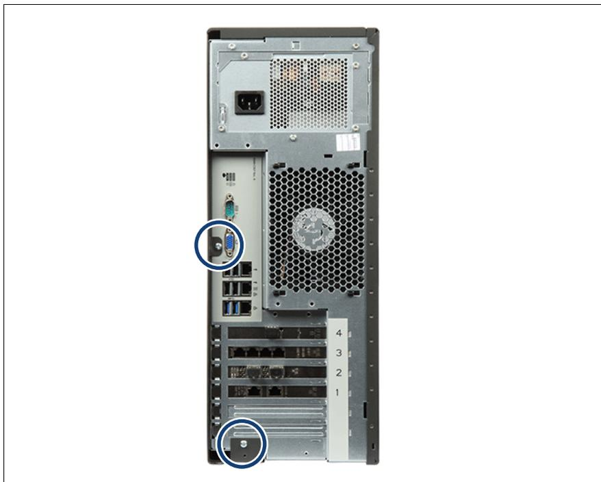
Figure 300: Removing the right side cover (A)
