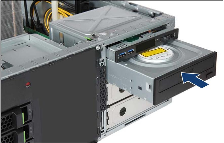
Figure 242: Inserting the accessible drive
