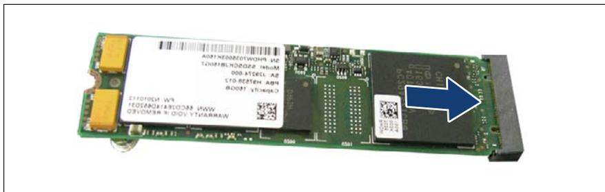
Figure 286: Installing the M.2 SSD
