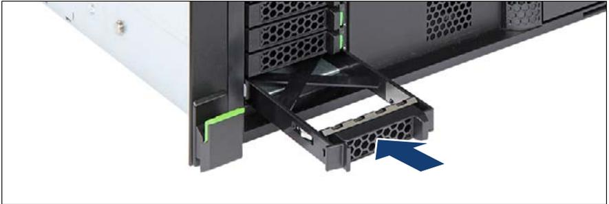
Figure 125: Installing a 2.5-inch HDD/SSD dummy module
