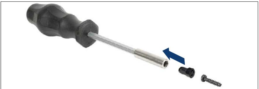
Figure 277: TPM bit insert
