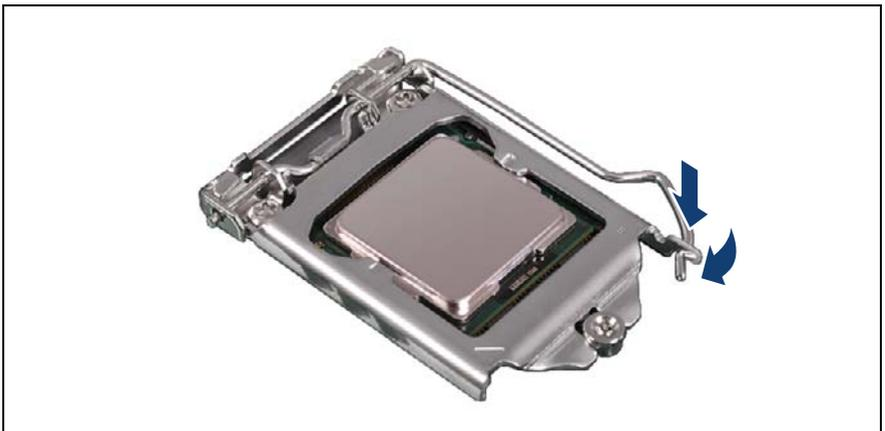
Figure 224: Closing the socket release lever
