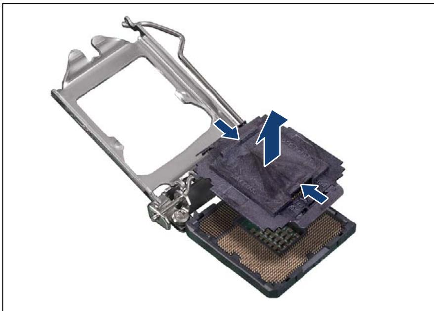
Figure 234: Removing the protective cover
