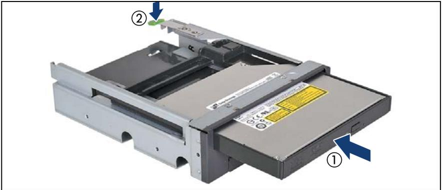
Figure 248: Mounting the slimline ODD module in the Multibay box
