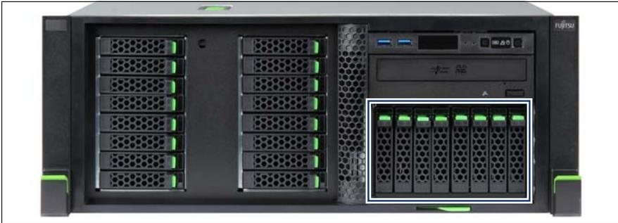
Figure 142: 8x 2.5-inch HDD/SSD extension box
