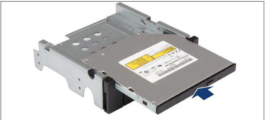
Figure 263: Installing the ultraslim ODD in the ultraslim ODD adapter (A)
