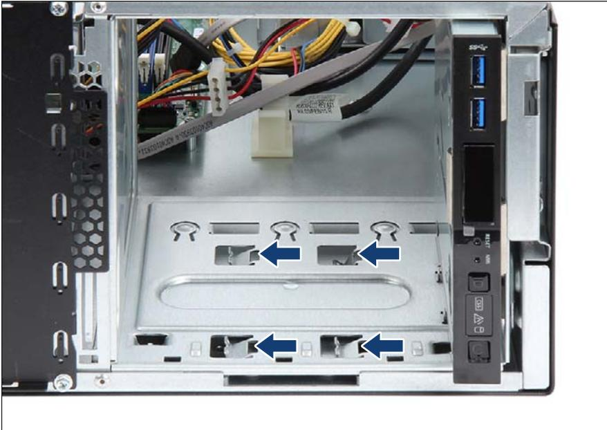
Figure 155: Bending in mounting brackets
