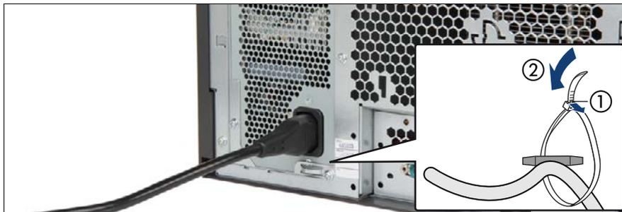
Figure 2: Unlocking the cable tie of a standard PSU
