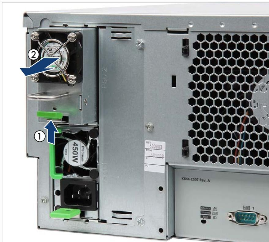
Figure 80: Removing a FJBU
