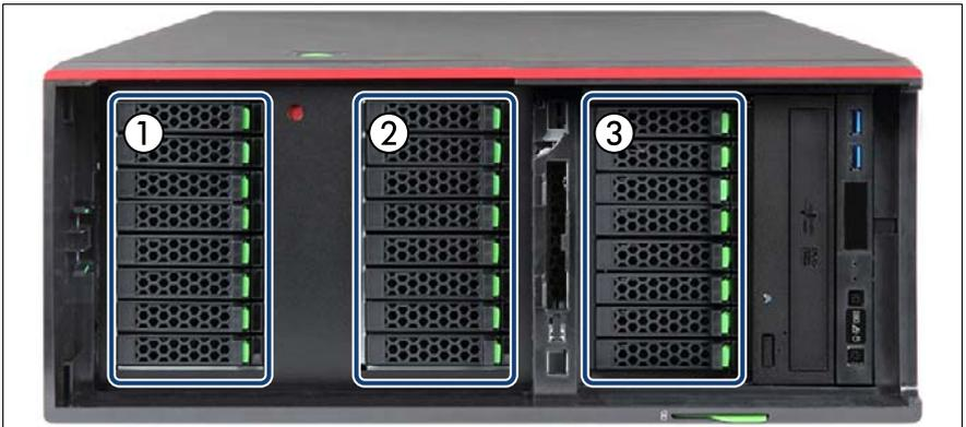
Figure 117: Example three backplanes - floorstand model
