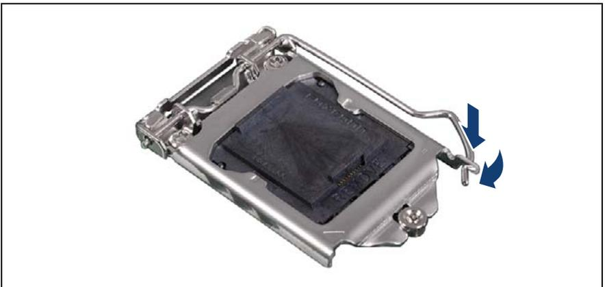
Figure 231: Latching the socket lever
