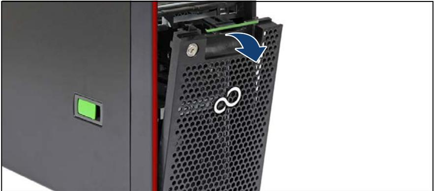
Figure 17: Removing the HDD bay cover
