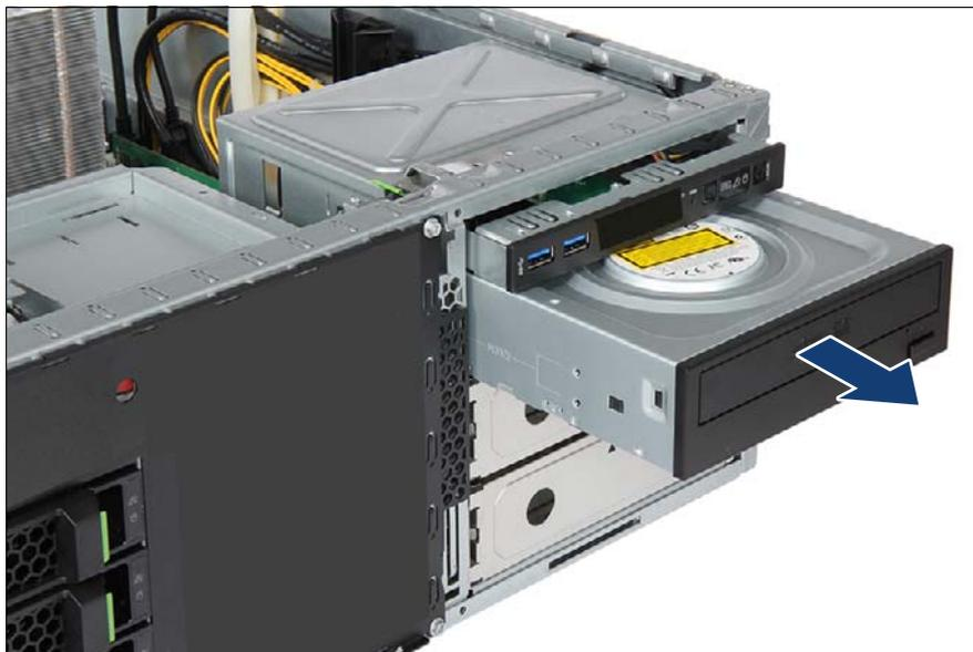
Figure 245: Removing the accessible drive
