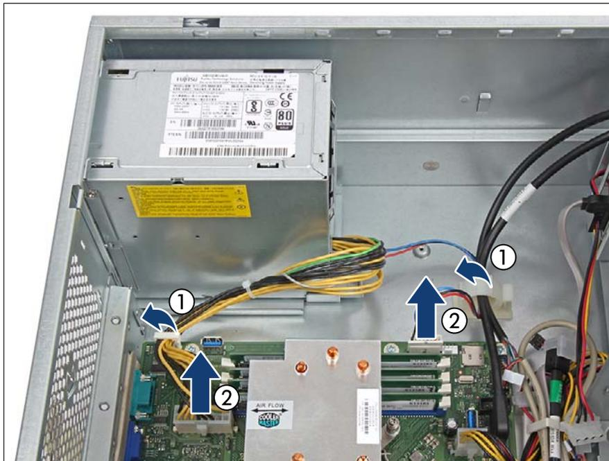
Figure 56: Disconnecting the power cables
