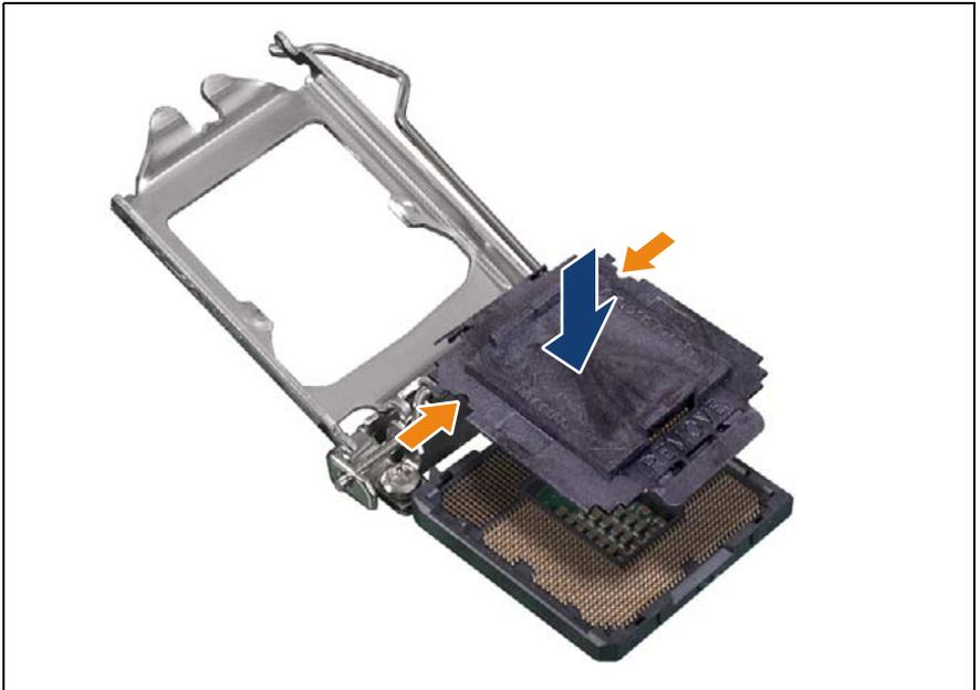
Figure 228: Attaching the protective socket cover
