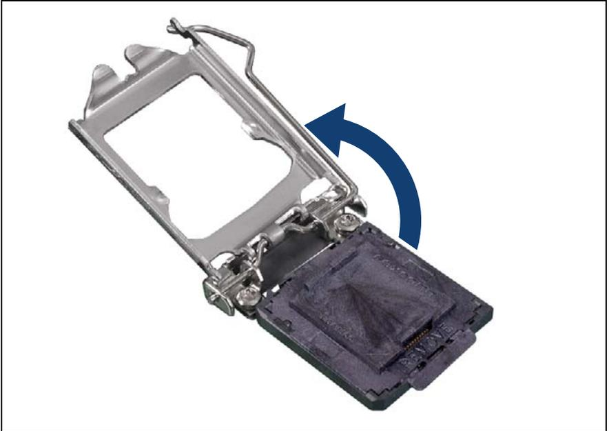
Figure 233: Opening the load plate
