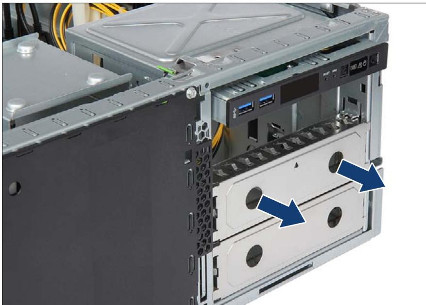
Figure 49: Removing an accessible drive filler cover
