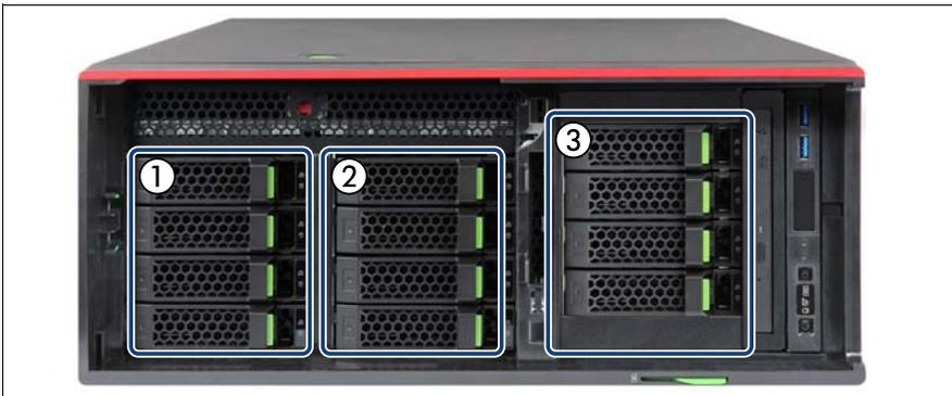
Figure 93: 3.5-inch HDD SAS backplanes - floorstand model
