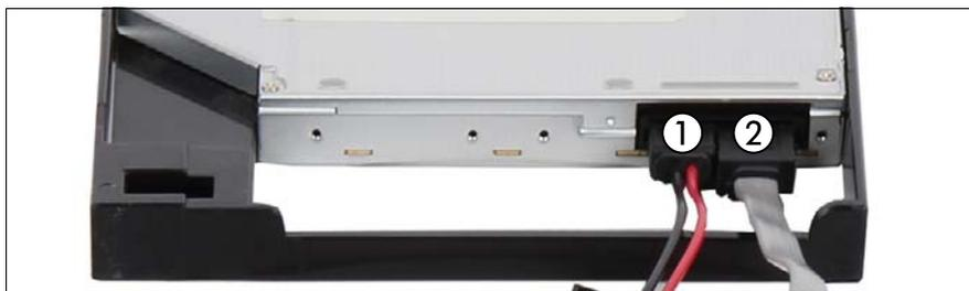
Figure 250: Connecting cables to the slimline ODD
