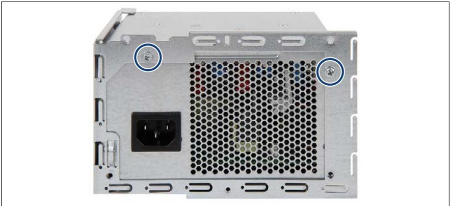
Figure 62: Securing the installation frame to the PSU
