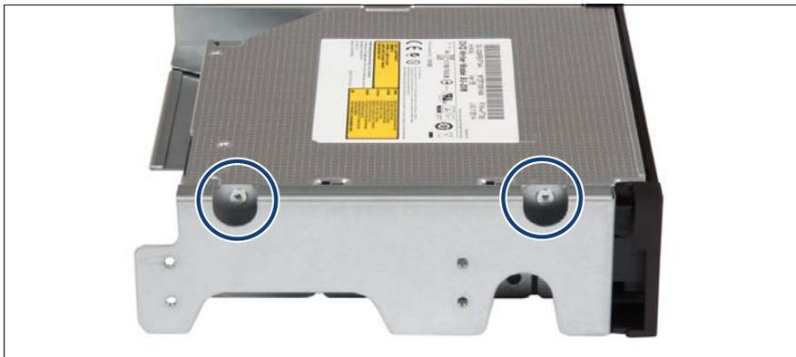
Figure 264: Installing the ultraslim ODD in the ultraslim ODD adapter (B)
