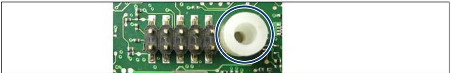
Figure 276: Inserting the TPM spacer on the system board
