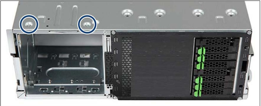
Figure 303: Detaching the accessible drive cage (A)
