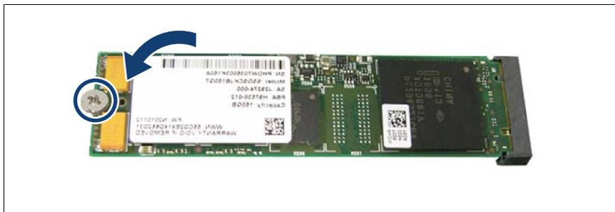
Figure 287: Fastening the M.2 SSD
