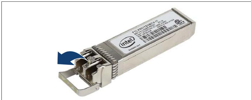
Figure 182: Unlatching the locking bail
