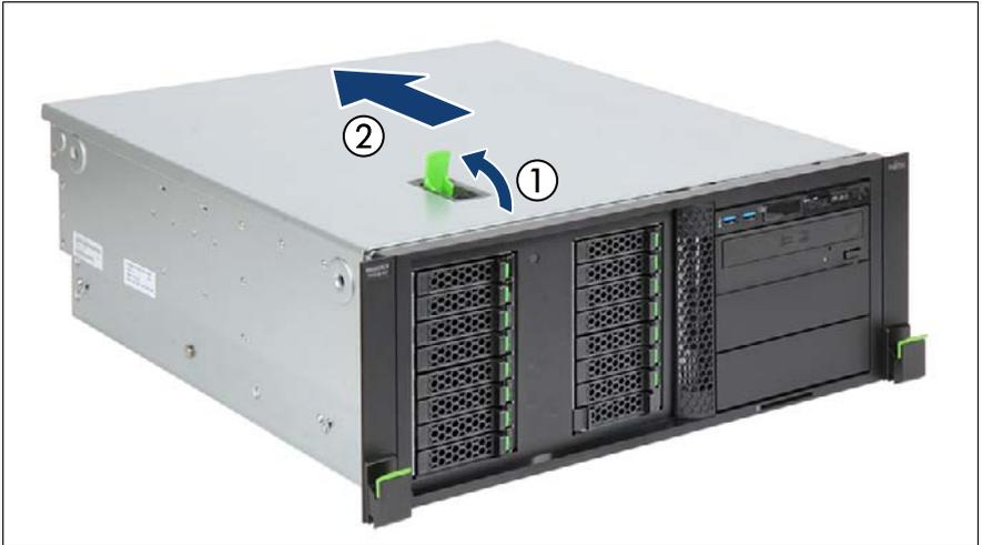
Figure 6: Removing the top cover (rack server)
