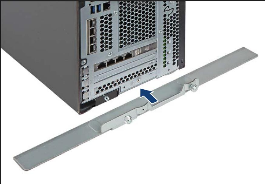
Figure 53: Installing the anti-tilt bracket (A)
