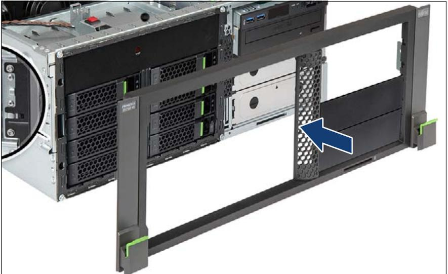
Figure 20: Installing the rack front cover
