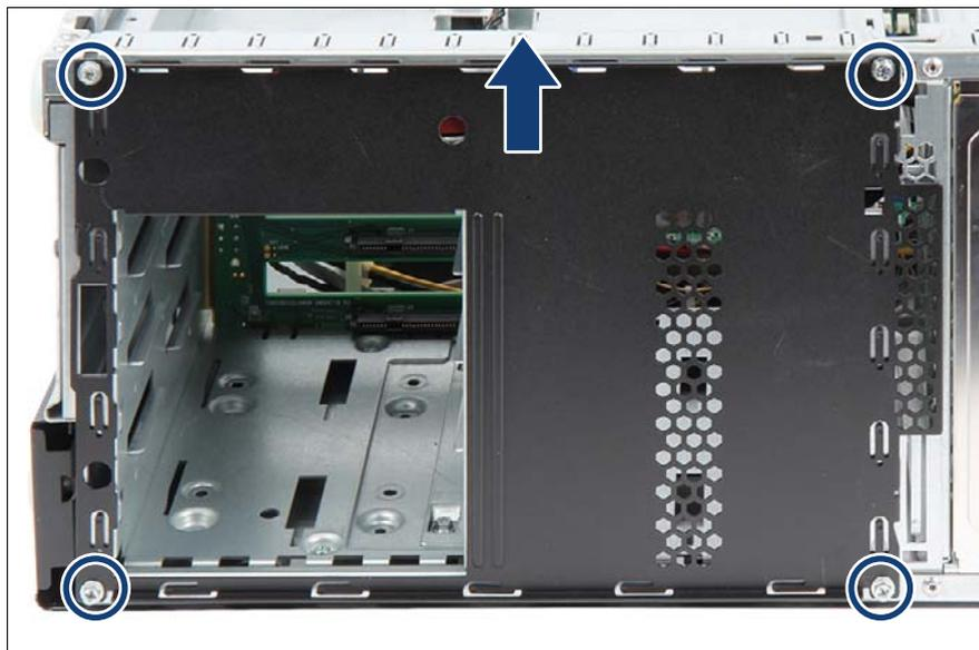
Figure 112: Removing the 4x 3.5-inch HDD front panel
