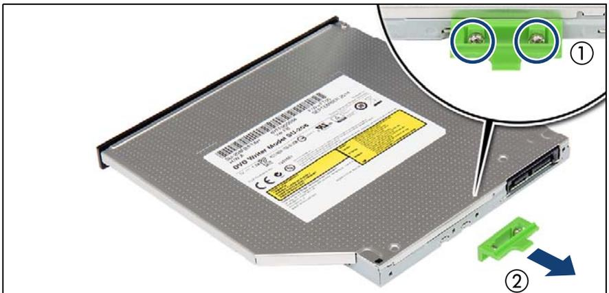
Figure 261: Removing the locking latch from the ultraslim ODD
