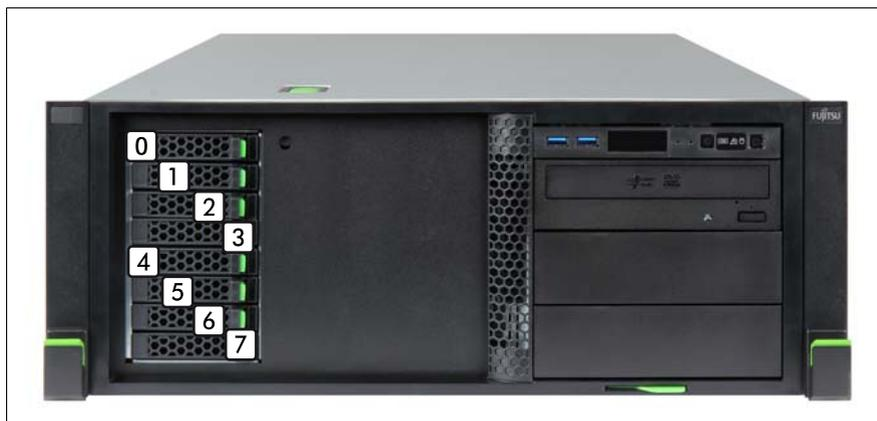
Figure 118: Configuration with up to eight 2.5-inch HDDs/SSDs
