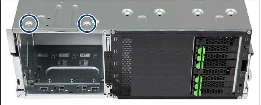
Figure 309: Securing the accessible drive cage (B)
