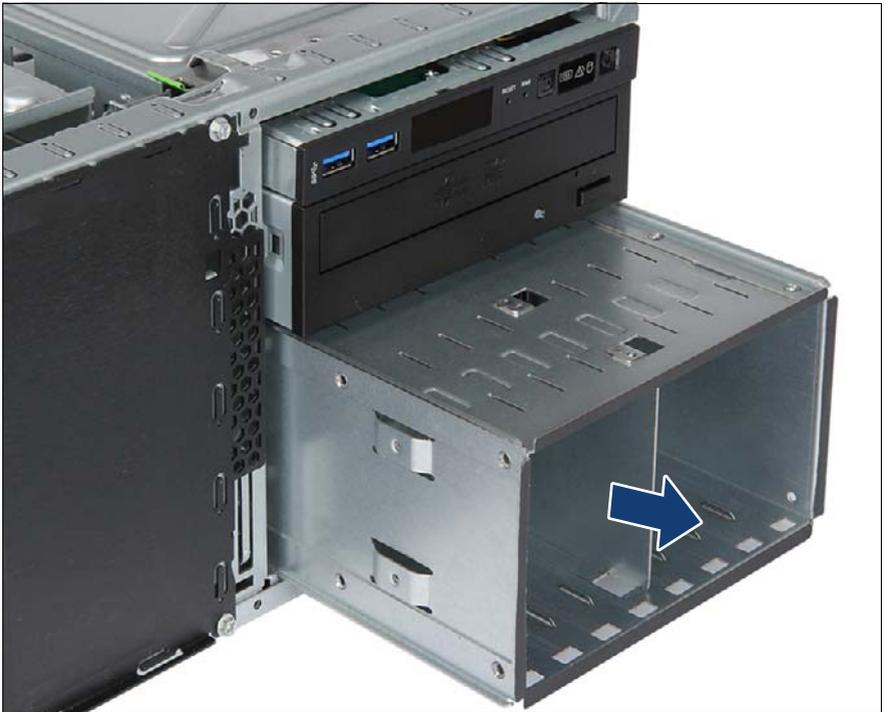
Figure 148: Removing the 8x 2.5-inch HDD/SSD extension box
