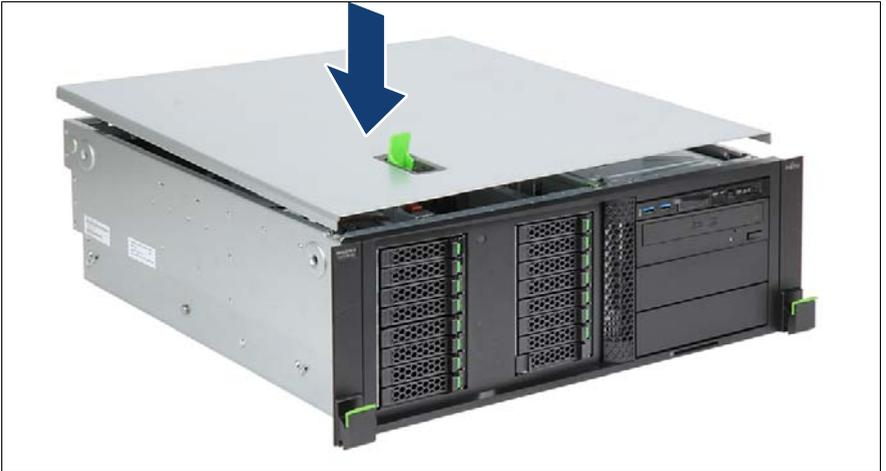
Figure 23: Installing the top cover (rack server) (A)
