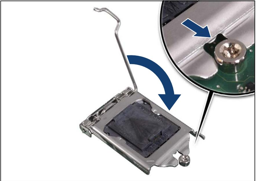
Figure 230: Closing the load plate (B)
