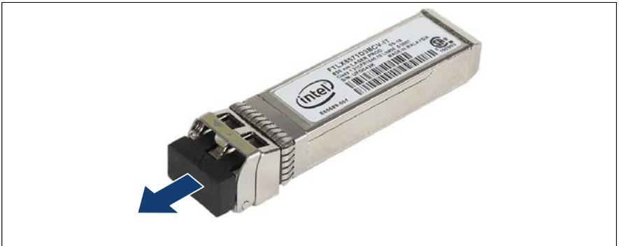
Figure 181: Removing the protective cap
