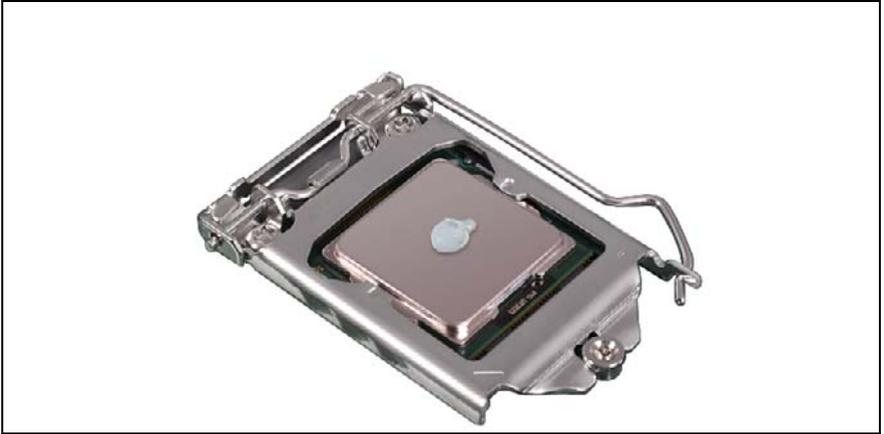
Figure 226: Applying thermal paste
