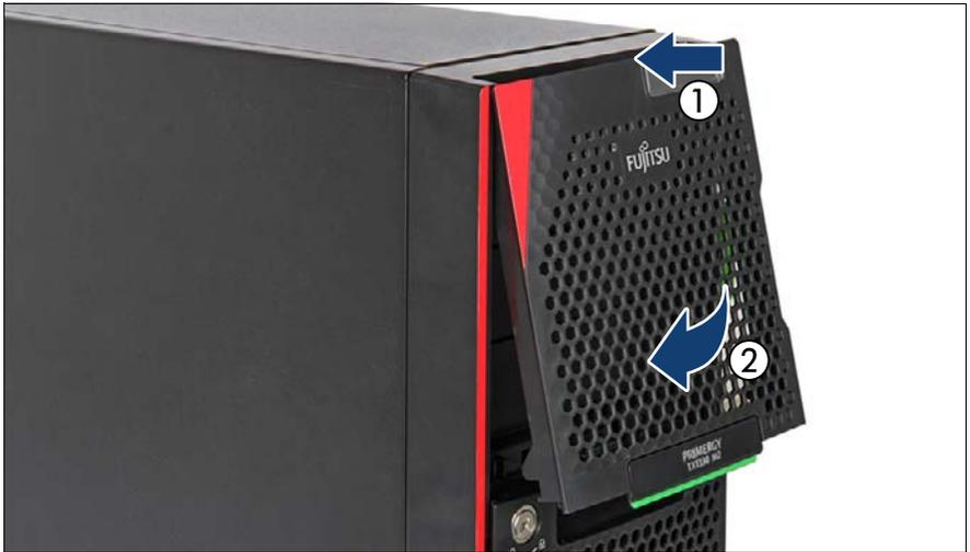
Figure 31: Installing the accessible drive bay cover
