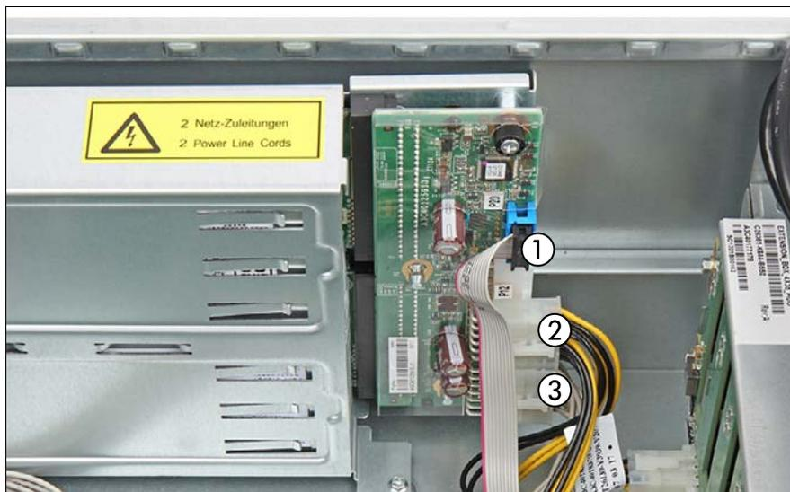
Figure 78: Connecting the power distribution board
