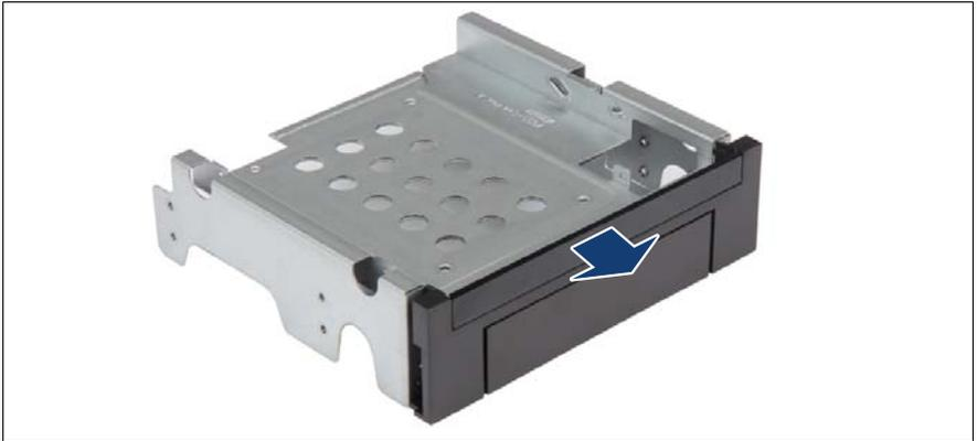
Figure 262: Removing the ultraslim ODD dummy cover - ultraslim ODD adapter
