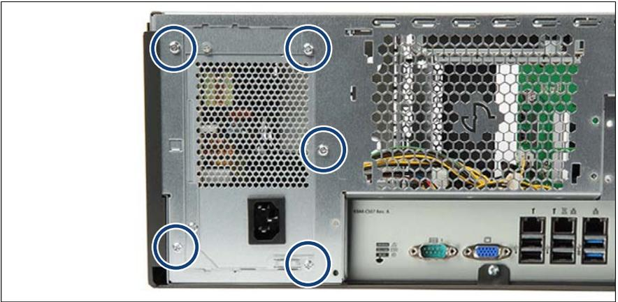
Figure 57: Removing the screws
