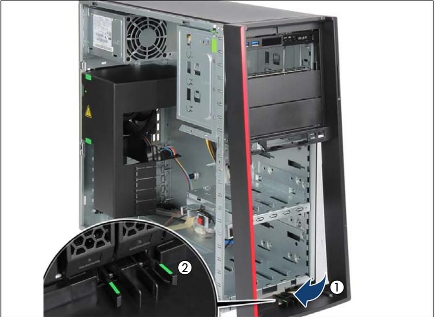
Figure 28: Installing the front cover (B)
