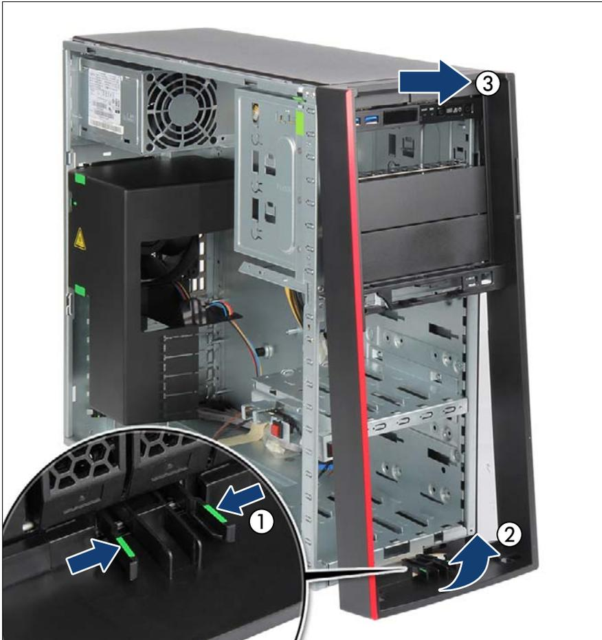
Figure 19: Removing the front cover (floorstand model)
