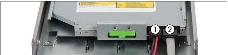
Figure 259: Connecting cables to the ultraslim ODD
