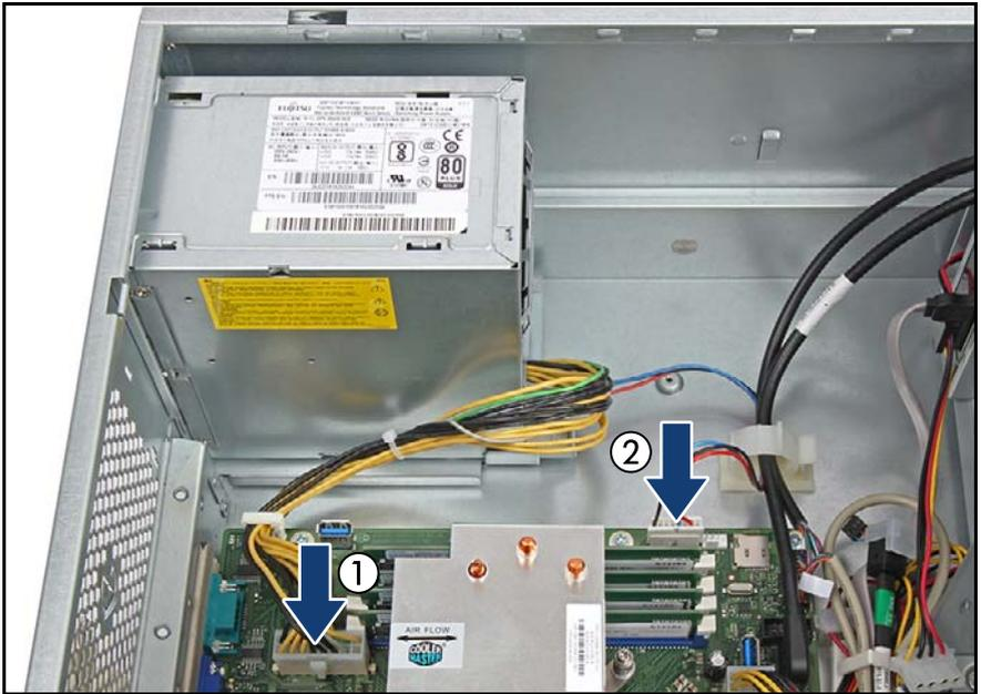
Figure 64: Connecting the power cables
