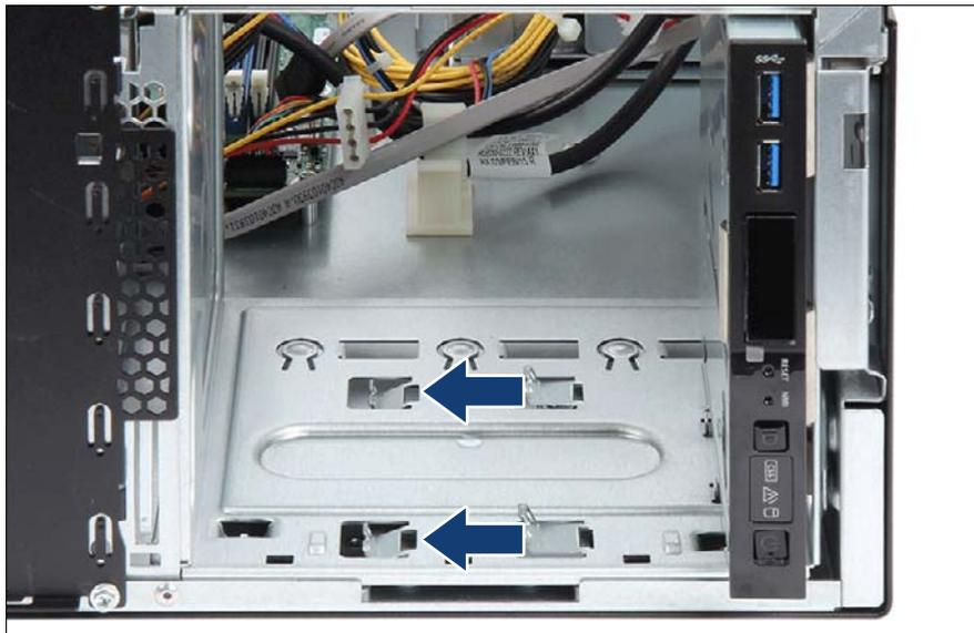
Figure 144: Bending in mounting brackets
