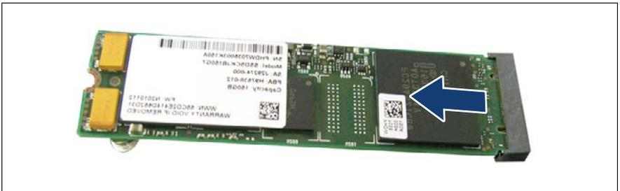
Figure 289: Removing the M.2 SSD (B)
