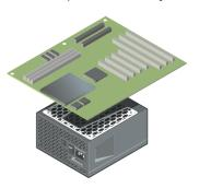
In general, it is recommended to mount the PSU with the ventilation top cover facing the motherboard. Due to the different varieties of case designs and layouts, however, please also consult the case manufacturer's instruction manual for additional information.
