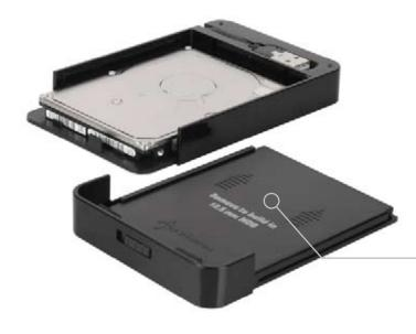
Using the adapter plate allows installing hard disk drives with 9.5 mm height.
