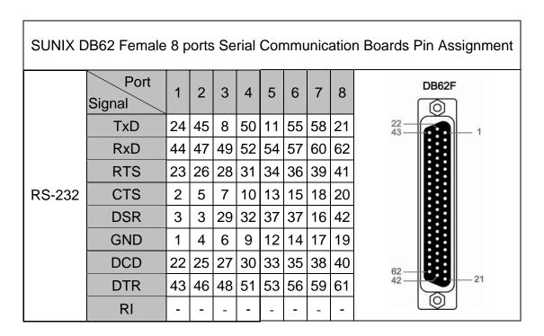
SUNIX 8-port RS-232 Low Profile Card builds DB68F connector on board.
