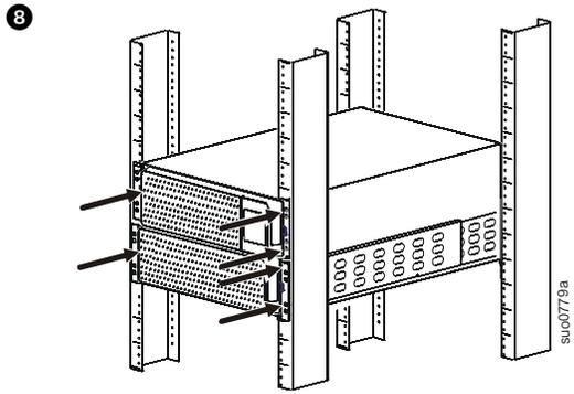
The process for installation of an external battery pack with UPS models SRT8K/SRT10K models is identical to that described for the SRT5K/SRT6K models.
