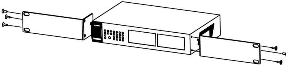
**Figure 13** Attaching the Mounting Brackets (GS1100-24)
