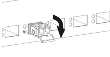
**Figure 10** Transceiver Removal Example
