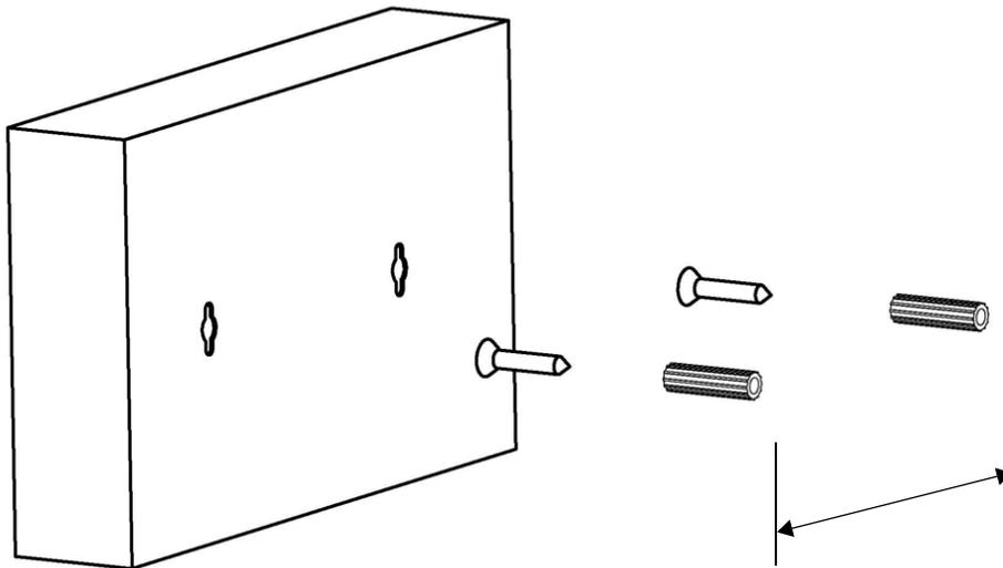
**The Switch should be wall-mounted horizontally. The Switch's side panels with ventilation slots should not be facing up or down as this position is less safe.**
