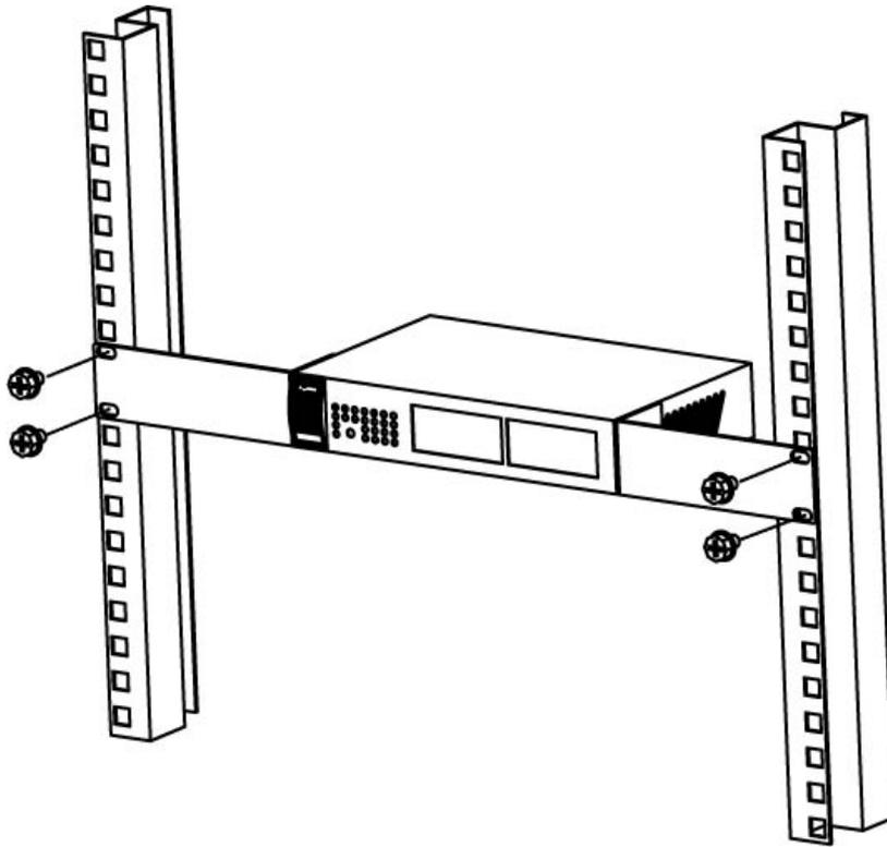
**Figure 15** Mounting the Switch on a Rack (GS1100-24)
