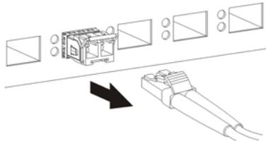
**Figure 9** Opening the Transceiver's Latch Example
