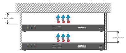
To prevent airflow restriction, we recommend allowing *at least* 1.75 inches (4.45 cm) of clearance between the top of your unit and the mounting surface. More space may be required depending on your environment.
