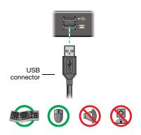
Note: To use a keyboard with your unit before your operating system starts, connect the A USB connector of your interface card to your computer (see "Connect your USB cable", page 12), and connect your keyboard to the USB connector labeled with a keyboard icon ( ) at the back of your unit.
