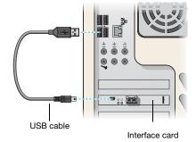
Note: To use a keyboard with your unit before your operating system starts, the USB cable must be connected from your interface card to your computer. Also, to use the audio hardware of your unit after your operating system has started, this cable must be connected.
