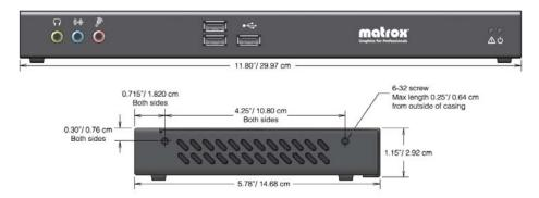
The mounting holes on the unit are 4.25 inches (10.80 cm) apart. Use four 6-32 screws. These screws can enter the casing by a maximum of 0.25 inches (6.35 mm).
