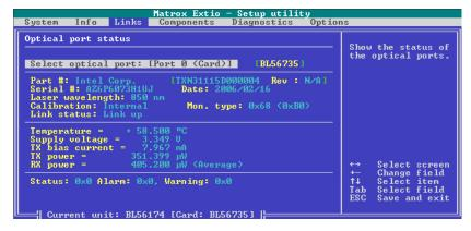
If you have multiple interface cards installed in your system, you need to change the Extio unit to view a different connection link.
