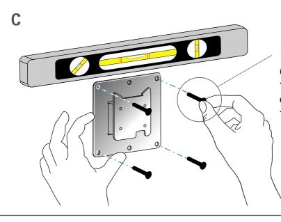
**NOTE:** Fasteners are not supplied. Consult a qualified construction professional to determine the appropriate type and quantity of mounting fasteners required for your application.
