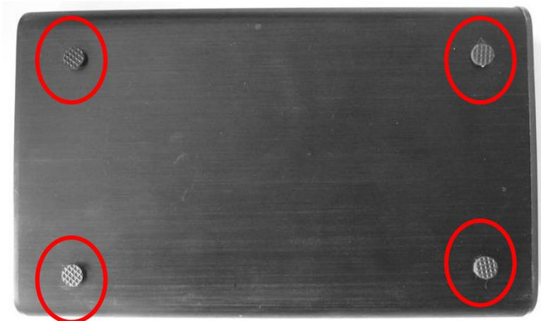
You can use the stand for vertical positioning. If you want to use the device horizontally, please mount the enclosed rubber feet at the bottom of the case.
