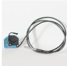
Temperature sensor connection to the module
