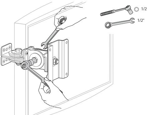
Side-to-Side Motion Move monitor side-to-side through entire range of motion. If it does not stay in place at any point it will need adjustment - see below. Adjust so side-to-side in place at any point it will need adjustment - see below. Adjust so side-to-side moving forces are equal.
