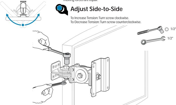
Portrait/Landscape Rotate monitor from Portrait to Landscape through entire range of motion. If it does not stay in place or movement in one direction is stiff tension poods. it does not stay in place or movement in one direction is stiff, tension needs adjustment - see below. Adjust until monitor stays in place and tension, portrait to landscape, is equal.
