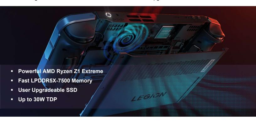
For cooling, the Legion Go utilizes an efficient fan that draws cool air through the back of the generously perforated galvanized steel backing and out through the top vents. In its highest performance settings, it's able to support up to 30-Watts of TDP.
