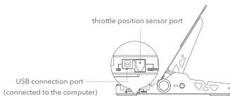
3. You will see the status of the SRP pedal in the Pit House once the wires are connected and the USB cable is plugged into the computer. (If it remains gray or does not respond, please unplug the USB port on the PC, turn off the MOZA Pit House, reconnect the USB port and turn on the MOZA Pit House)
