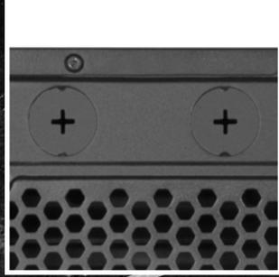
Installation opening for CPU coolers
