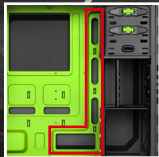
Cable management system
