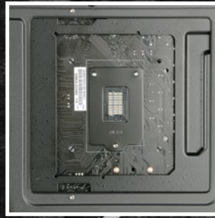
Installation opening for CPU coolers
