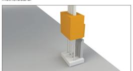
Position the cooler over the CPU.
