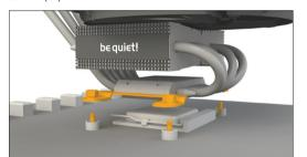
and affix by turning the AMD M3x15 screws (10) from the rear side of the motherboard.
