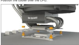
Place the hexagonal nuts (8) over the spacer nuts (7) and progressively tighten these in a crosswise manner until firm using the hexagonal wrench (14).
