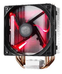
Hyper 212 LED is equipped with PWM Fan with red LEDs and provides the best airflow and static pressure to take the heat away. And four direct contact heat pipes with funnel shaped aluminum fins provide the optimized CPU coolers for great performance. Moreover, the improved universal bracket designs ensure easy and worry free installation on all platforms.
