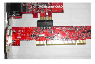
Install the adapter card into a PCI slot on the motherboard and secure the bracket to the computer case.
