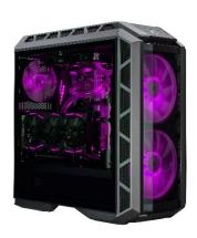
Clear View Inside – The MasterCase H500P has a light grey tinted tempered glass side panel and plastic top/front covers, making it ideal for showcasing your build with (RGB) lighting.
