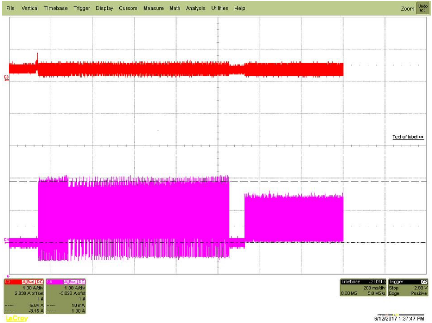
Figure 1. 12TB - Typical 5V and 12V startup and operation current profiles
