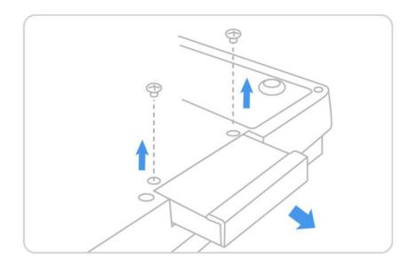
**Step 4-** Attach drive bracket to the new Solid-State Drive. Slide the drive into the bay until fully seated (Make sure to align the SATA plugs and solid state drive connectors).
