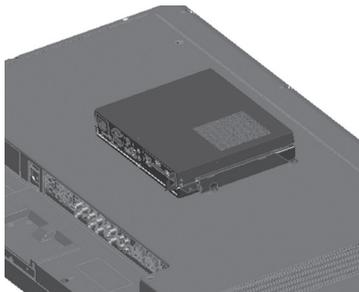
6 Use screws to secure the player and the Box Guide as shown below.
